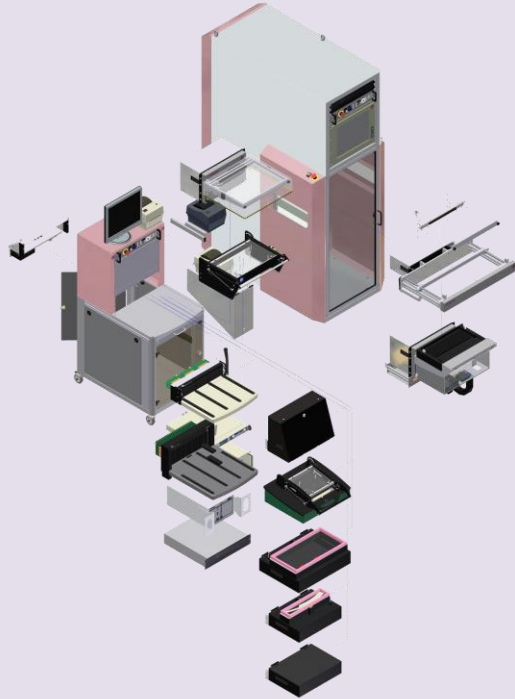
Modularity. 6tl modules fixed into a 19" rack to integrate into a standard testing platform
