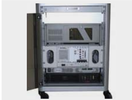
Enough free space for installing 19 inches instruments.
