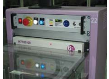
Operator interface module including navigation keyboard, display and start, stop and emergency push buttons.
