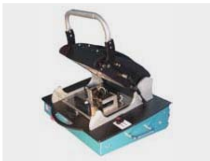
Fixture 7200.7110 with a Faraday mini chamber to test RF receivers
