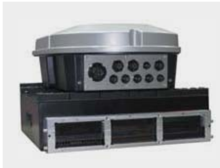
Fixture 7200.7310 including transports rollers for final test of assembled products.
